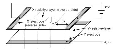
Vcc = 5.0V**Output Data** χl A in 0V 0000h (Min.) Α В 1.25V 00FFh 01FFh С 2.5V D 3.75V 02FFh Ε 5V 03FFh (Max.)
