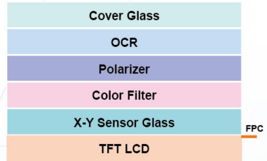
TED Structure Sensor mounted on top of TFT LCD
