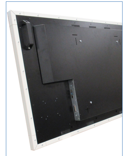
Backside of Brilan 4K 54.6, including glass protection frame in white
