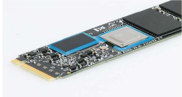
A mechanical bond is applied around the key components
